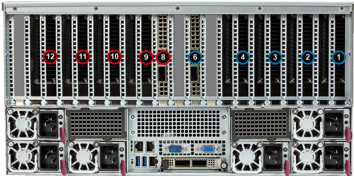
Figure 3-22. AS -5126GS-TNRT Expansion Card Slots
